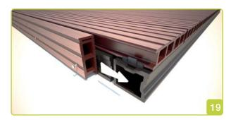
Fixing the Edenex Plank as a skirting board is relatively simple. Screw through the plank, into the Edenex plank edge with no more than 500mm between fixings using screws long enough to engage the second rib on the deck plank. Fig 19.
