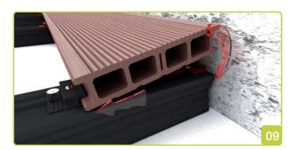
Position the decking plank, so that it fully engages in the fixed Centre Clip. Then, push the decking plank downwards as shown in Fig 9. This will engage the clip action of the end clip, and the plank will lock into position.
