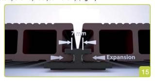
To allow for expansion use spacers cut to 7mm to check that a 7mm space is maintained between planks running parallel. Over a period of time the planks will expand to close this gap to approximately 4mm. (Fig 14-2). Expansion room is allowed for in the new centre clip as shown in
