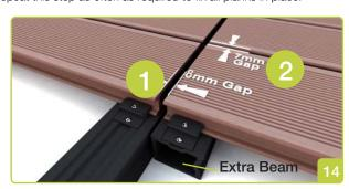
When placing planks end to end it is important to allow a minimum of 8mm between planks. This distance will slowly close as the planks expand. (Fig 14-1).
