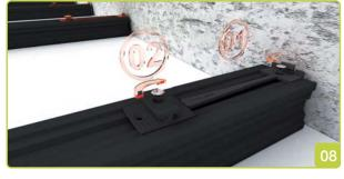
Starting at the top, place the End Clip into the groove on the Support Beam and secure in place ensuring that the end of the clip with the screw hole is flush with the edge of the support beam as shown in Fig. 8 - 1.
