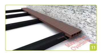
If the Edenex plank finishes parallel to a wall or structure, it is essential to leave a gap between the plank and the wall. Allow a 4mm gap along the length and a 10mm gap at the end (Fig 12).
