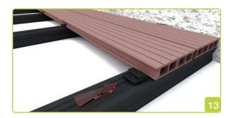
From here, the process is very straightforward. Position the next decking plank into position, by again, engaging it in the fixed Centre Clip as shown in Fig 13. Use this board to position the next clip and screw into place. Repeat this step as often as required to fix all planks in place.
