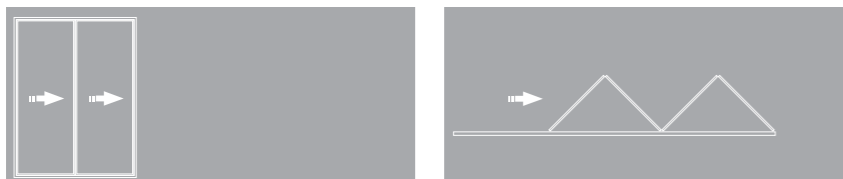
TWO PANE CONFIGURATION (2 panes, 2 sliding, 0 swing)
