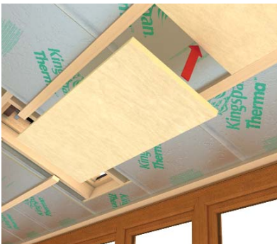
Install insulation between batten
