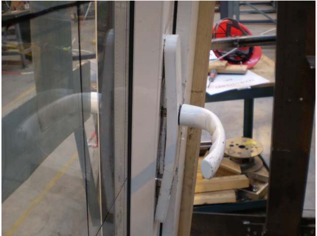
Damage to the handle following basic security test
